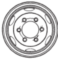
Bolt hole to bolt hole. Causes: Loose cap nuts, small hub backup (also see bolt hole cracks/distortions).
