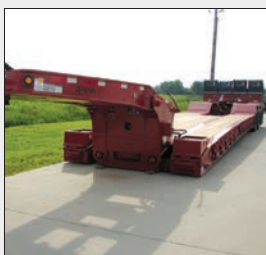
heavy-duty outriggers upper flange reinforcement
